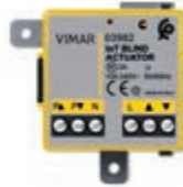
03982 Actuator for 1 roller shutter with slat orientation and change-over relay output for cosφ 0,6 motor 2 A 100-240 V~ 50/60 Hz, remote control, Bluetooth® wireless technology 5.0 for View Wireless mesh system and Zigbee 3.0
