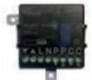
03996 Centralizable relay module, slat orientation, with relay outputs for cosφ 0,6 motor 2 A 220-240 V~ 50/60 Hz, position saving, for backside or junction boxes installation
